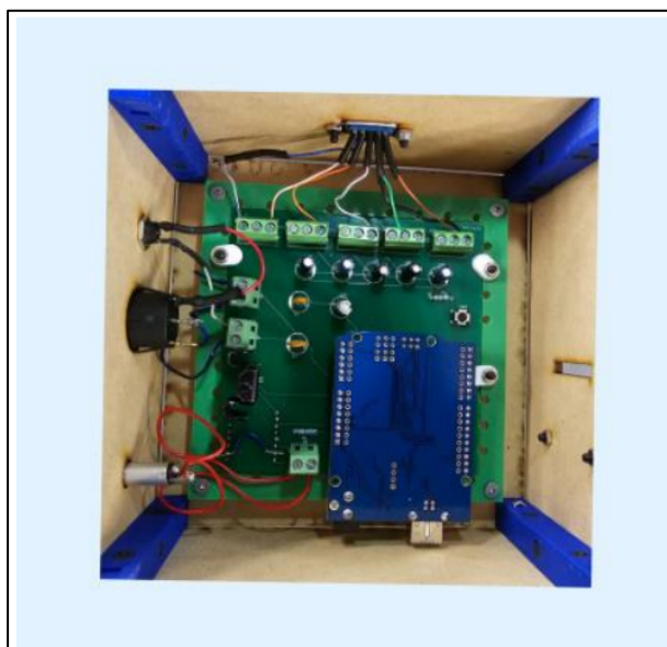
Figure 5. Assembled electronic board with all components required to display audible information.
